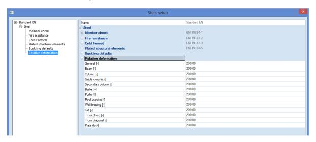
With the option "Steel -> Beams -> SLS Checks - Relative deformation", the relative deformations can be checked. The relative deformations are given as absolute value, relative value related to the span, or as unity check related to the limit for the relative value to the span.
