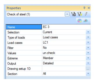
The selection is set to 'Current' to only see the results of the selected member (column B4). The flexural buckling check will be performed in the **Stability check** and can be shown in the 'Detailed' output.
