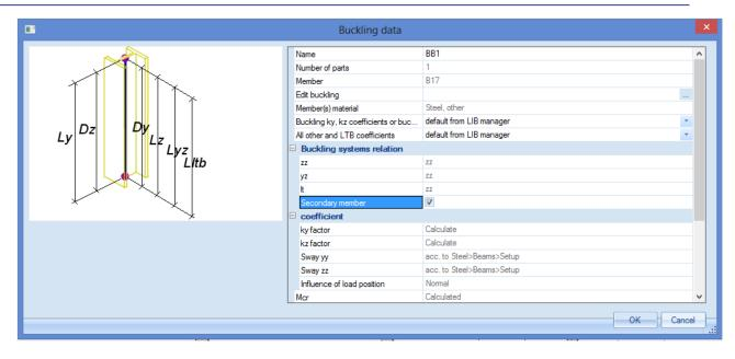
Afterwards, a label will be displayed on beam B17, indicating that this beam consists some buckling data. This buckling data is **Additional data** and can be copied to other members in the structure.
