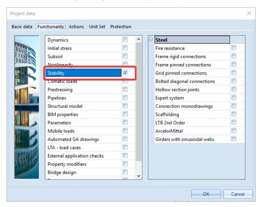
2) Create a Stability combination. This can be done in the service Load cases, Combinations => Stability combinations. In this example, the combination factor is kept equal to 1 with the consequence that the calculated critical load factor  $\alpha_{cr}$  will be equal to the critical Euler force  $N_{cr}$ . This will be explained in one of the following steps.
