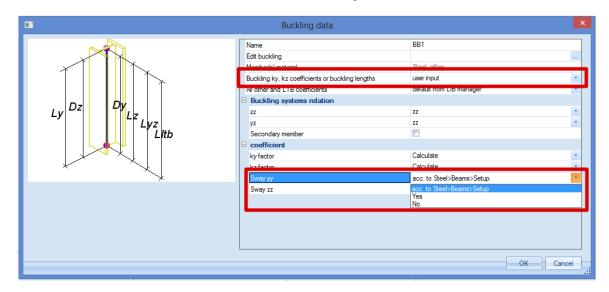
The option 'Buckling ky, kz coefficients or buckling lengths' has to be set to 'user input'.
