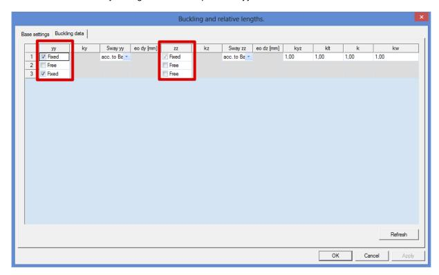
These settings will be stored in the buckling system BC\*. This buckling system can be used for other elements, but only of these elements do have the same amount of structural nodes.
