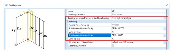
**Remark:** As mentioned in Step 2) the stability analysis calculates the critical load factor  $\alpha_{cr}$ . This value can be used to determine if a structure can be designed with a first order analysis or need to be designed using a second order analysis taking into account global and or local imperfections as described in EN1993-1-1 article 5.2.1(3):
