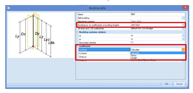
First of all, the **Buckling ky, kz coefficients or buckling lengths** has to be set to **user input**. Next for the ky factor, there are three possibilities:
