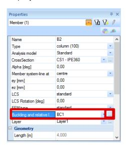
By clicking on the three dots, the 'Buckling data' window will open. After clicking on 'Edit', the sway type can be changed.
