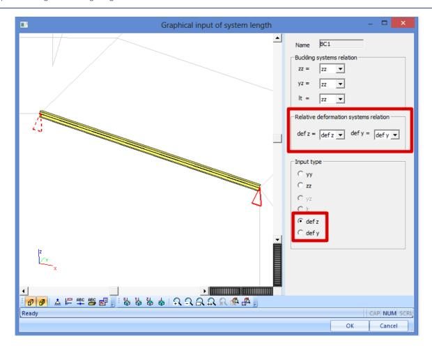
The relative deformation is always regarded according to the local axis of the member. For the deformation in the y direction of the member, there are two supporting nodes for member B3. The distance between these nodes is 6,083m.
