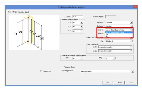
These settings are stored in the 'Buckling system' BC1. This system can be used for other members, if these members have the same amount of construction nodes.
