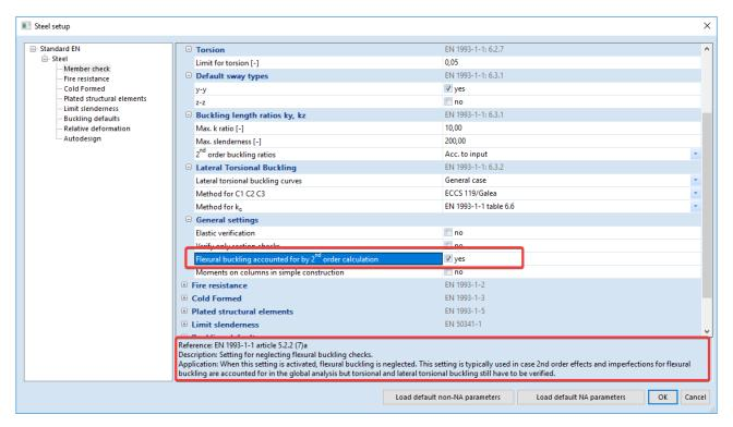
By activating this option, SCIA Engineer will take the buckling ratios ky and kz equal to 0,001. This neglectable buckling ratios will influence the following two stability checks which are described in EN1993-1-1:
