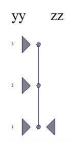
When looking at the rendered view of the structure, it is clear that beam B17 is too weak to have an influence on the system length of column B3. In SCIA Engineer, there is a possibility to exclude a beam from a buckling system. This can be done by inputting **Member buckling data** to the element.
