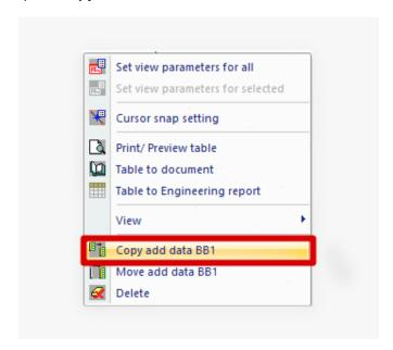
If the additional data (secondary member) is inserted, the buckling system of column B3 can be changed.
