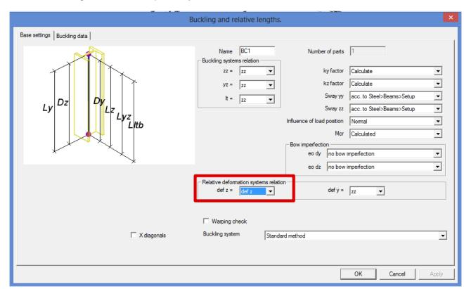
This can be changed to create a separate system for the relative deformation.
