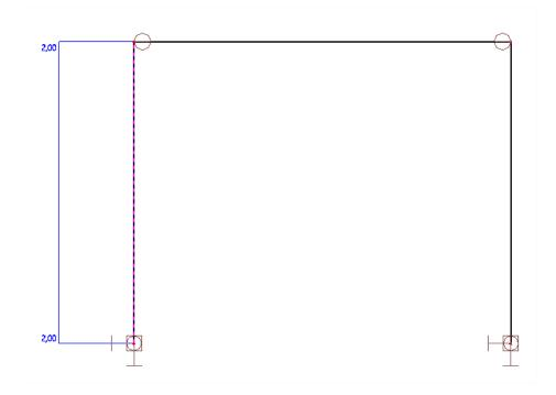
**Note**: If the buckling ratios are calculated automatically, by default a maximum value of 10 is used. This limitation can be adapted in the Steel setup.
