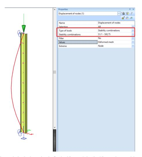
The result clearly shows that the first buckling mode is a buckling mode around the weak z-axis (as expected). As a consequence, this buckling mode can be used for the calculation of the buckling ratio  $k_z$ . The same can be done for the buckling ratio  $k_y$ . In this particular example, the forth buckling mode is the decisive one for the strong y-axis buckling.
