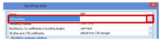
In the next window, the buckling ratio ky or the buckling length ly can be inputted.
